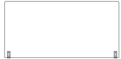
ile 241 S w 2500 x h 1250 x d 512mm w 98,43 x h 49,21 x d 20,15"
